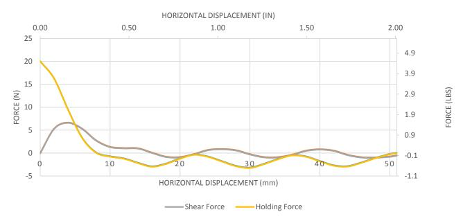
When two 1000587 Polymagnets are laterally offset their attractive force decreases while their centering force increases. The magnets will have minor detents and a relatively low holding force when they are offset. This feature can be incorporated into a system to give feedback to the user during an assembly process.
