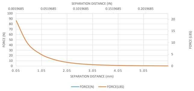
These Polymagnets provide very strong attachment forces to steel over their effective range compared to conventional magnets. These magnets are suitable for use with a metal target. The holding strength for these Polymagnets can be enhanced in many applications by using a thin steel shunt directly against the back of the Polymagnet, and this shunt will also help limit stray fields from the magnet.
