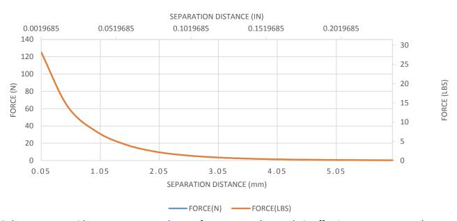
These Polymagnets provide very strong attachment forces to steel over their effective range compared to conventional magnets. These magnets are suitable for use with a metal target. The holding strength for these Polymagnets can be enhanced in many applications by using a thin steel shunt directly against the back of the Polymagnet, and this shunt will also help limit stray fields from the magnet.
