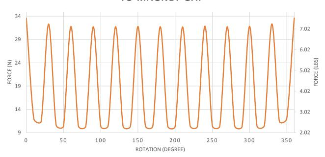
These Polymagnets provide an indexing feature. This aids in the assembly process as well as provides a flat surface to resist torque created as the magnets are rotated.
