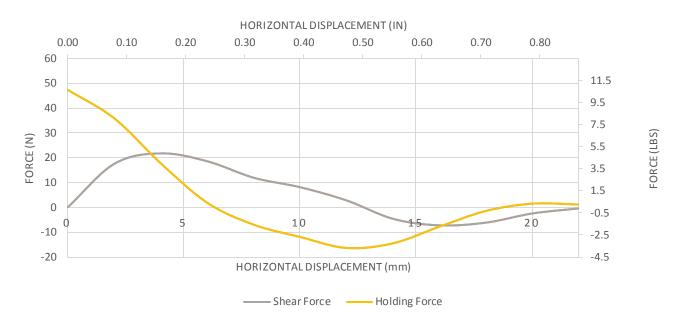
When a pair of 1002229/1002230 Polymagnets are laterally offset their attractive force decreases while their centering force increases. The magnets will have minor detents and a relatively low holding force when they are offset. This feature can be incorporated into a system to give feedback to the user during an assembly process.
