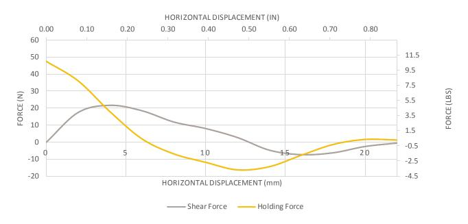
When a pair of 1002230/1002229 Polymagnets are laterally offset their attractive force decreases while their centering force increases. The magnets will have minor detents and a relatively low holding force when they are offset. This feature can be incorporated into a system to give feedback to the user during an assembly process.
