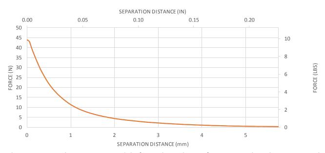
These Polymagnets provide very strong, tightly focused attachment forces to steel or their mating Polymagnet. These magnets are suitable for use with a metal target or another 1002237 Polymagnet.
